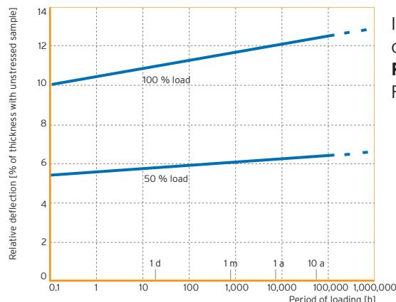
Increase in deformation under consistent loading
