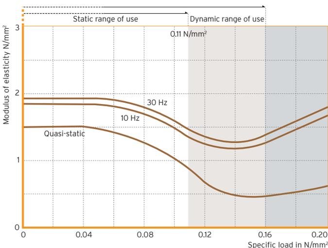
Fig. 3: Load dependence of the quasi-static and dynamic modulus of elasticity, using the example of Sylomer® SR 110
