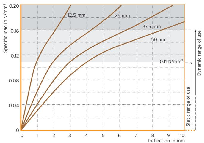
Fig. 2: Load deflection curve, using the example of Sylomer® SR 110
