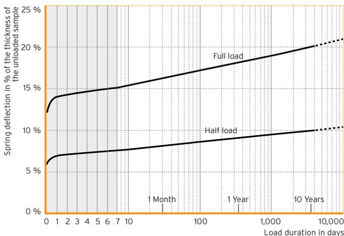
Fig. 5: Static long-term durability of Sylomer®
