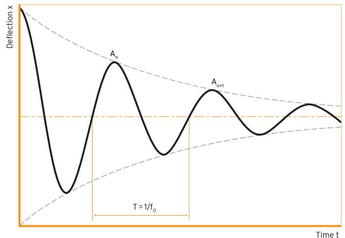
Fig. 8: Fading behavior of a free vibration displacement x
