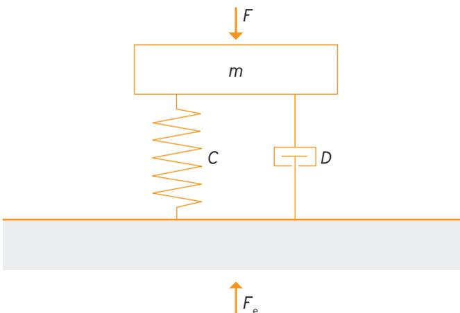
Fig. 7: One-dimensional mass-spring system
