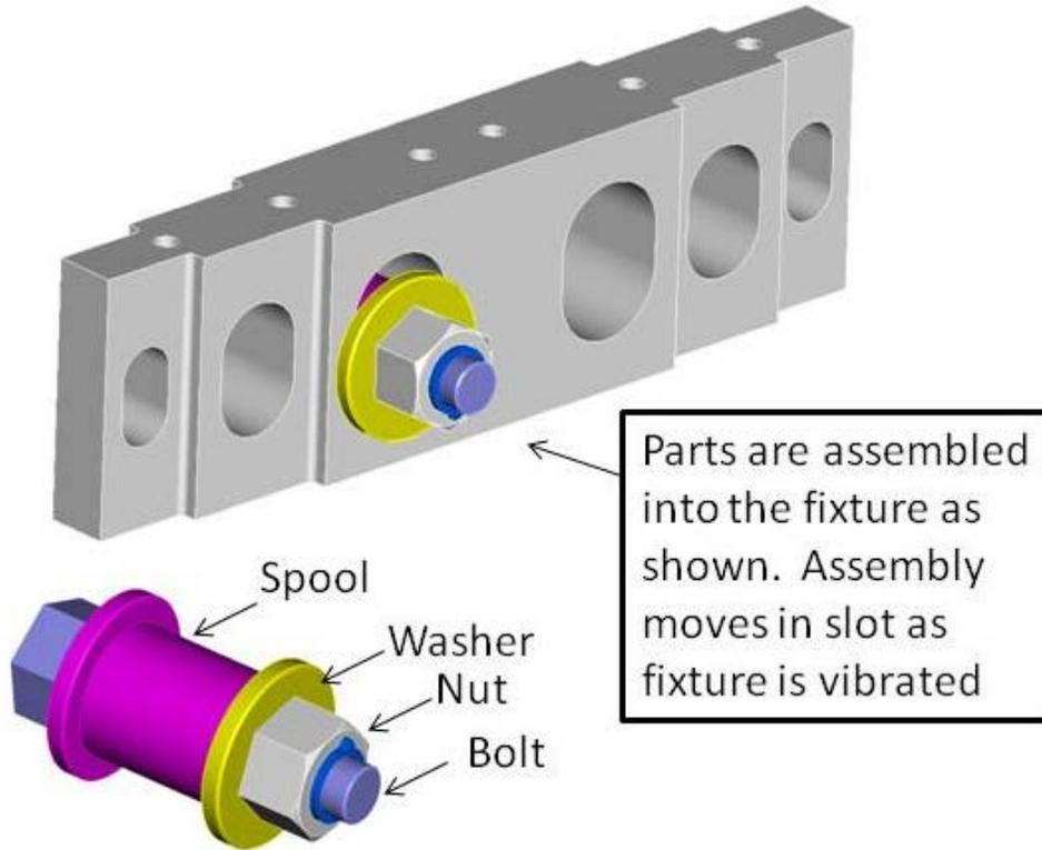
Picture of fixture used in vibration test
